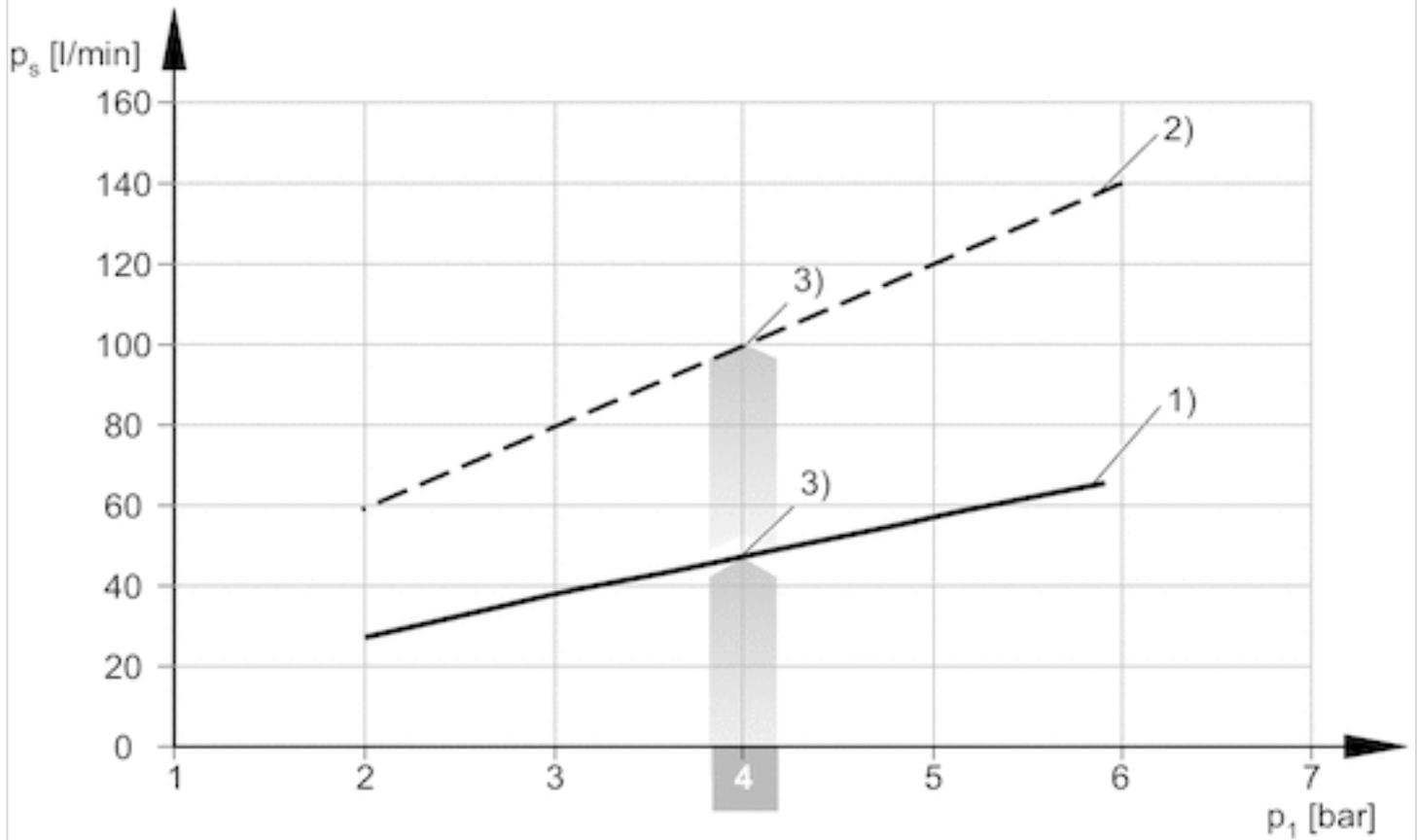
1) Ø buse 1.0 mm 2) Ø buse 1.5 mm 3) Pression de service optimale
