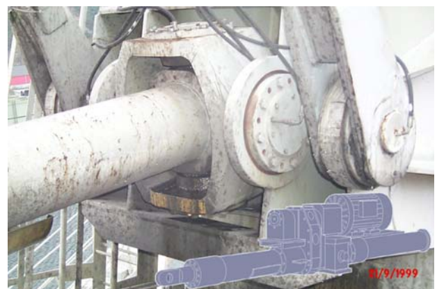
Fig. 03/04: Drive unit and cardanic mounting of the electromechanical spindle adjustment
