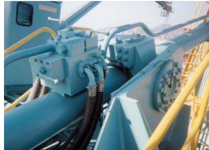
Fig. 13/14: The cylinder is safely locked in any position
