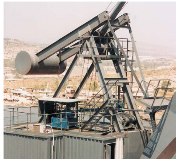
Fig. 24/25: The arrangement on the roof saves pipework, if only the luffing cylinder has to be supplied
