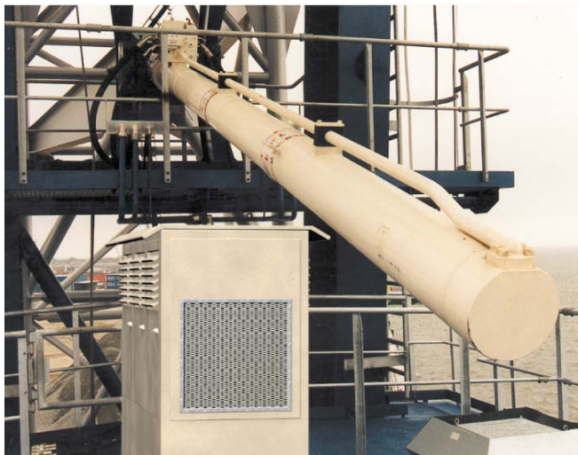
Fig. 24/25: The arrangement on the roof saves pipework, if only the luffing cylinder has to be supplied
