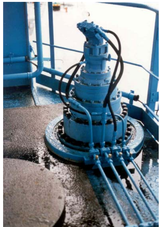
Fig. 18: Hydrostatic slewing drive with gearbox, brake and axial piston motor
