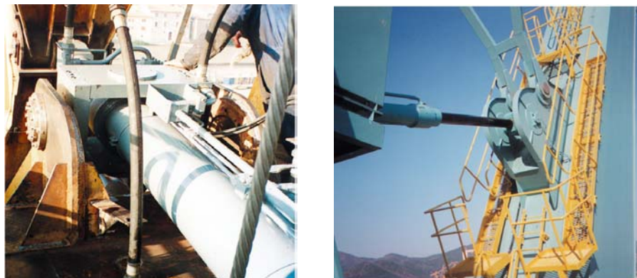
Fig. 06/07: The cardanic support and the mounting element of the eye are custom-made.
