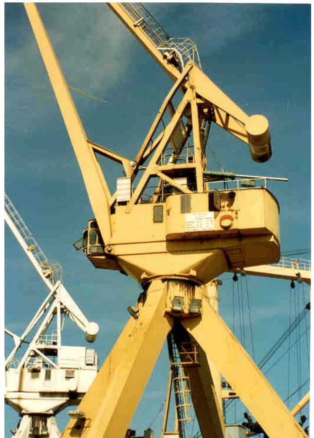
Fig. 02: Level luffing crane with double-rod cylinder in Koper / Slovenia
