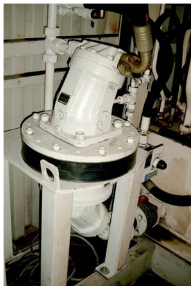
Fig. 09/10: Structure of a flow divider combination
